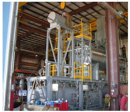
footprint than a comparable DOW azeotropic dehydration unit and, of course, several times more compact than a conventional Mole Sieve unit. And the high tech Azeo process, combined with high dewpoint depression Sulzer Structured Packing, is often more compact than conventional glycol dehydration unit. This saves plant area requirements and off-shore reduces weight support costs.
