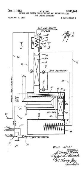
The introduction of a gas stripping column for polishing the glycol after reboiling allowed regeneration systems to attain a glycol purity of 99.9% for a resultant gas water content of under 4 lbs per MMSCF, which specification was а employed in areas with colder climates hydrate formation and water condensation in pipelines was more problematic.
