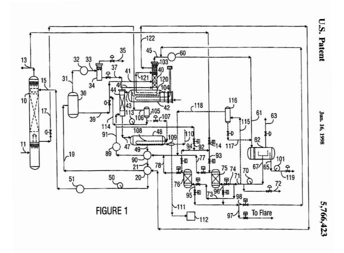
In 2005 work began on a modified DOW process whereby an improved and simplified method of azeotropic stripping and distillation of gas drying liquid desiccants was made possible.
