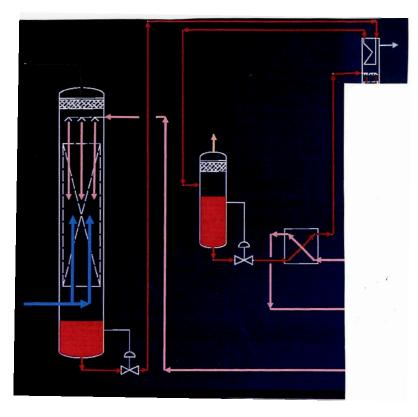
Rich liquid desiccant is level controlled from the contactor to the still column condensing coil of the reboiler, where the cooling effect of the relatively cold liquid desiccant condenses reflux water out of the distillation column overhead steam to minimize overheads glycol vaporization losses, and the now warm rich glycol then flows to the glycol flash separator absorbed soluble gases are flashed off.
