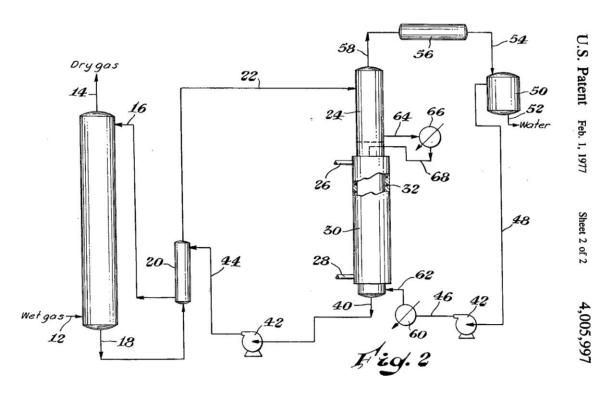
Again, the still column overheads were condensed, the liquid water was rejected and the condensed hydrocarbon liquid was pumped, vaporized and reintroduced to the stripping column. This process allowed regeneration systems to attain a glycol purity of 99.99% for a resultant gas water content in the low parts per million.
