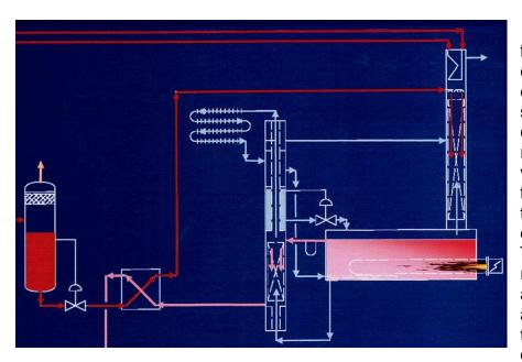
The rich glycol flows down the still column, which is equipped with a packed section, counterand currently contacts reboiled glycol and water vapors and the heat from said contact strips the water from the downflowing desiccant. The vaporized water rises up the still column is directed and to atmosphere or to thermal oxidizer or to an overheads condenser for
