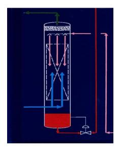
The drying of natural gas takes place in a high pressure gas/glycol countercurrent contactor with the relatively high pressure wet gas entering the bottom of the contactor and the dryed gas exiting the top. Lean or dry glycol enters the upper side of the contactor and rich or wet liquid desiccant exits bottom of the the contactor.
