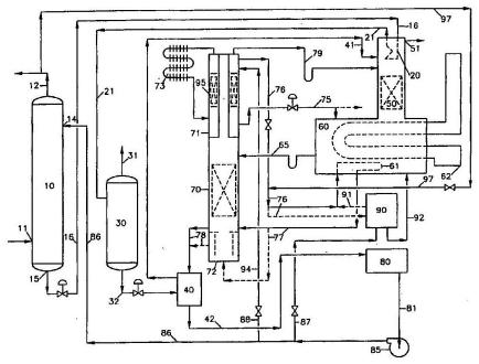
This thermally driven octane recycling percolation system eliminates pumps and simplifies other systems required in the previously described azeotropic processes and eliminates the venting of methane stripping gas that has become so environmentally problematic in the Stahl process.
